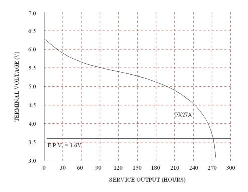
DISCHARGE METHOD: 20k ohm ; 24 hours/day TEMPERATURE: 20+/-2°C
