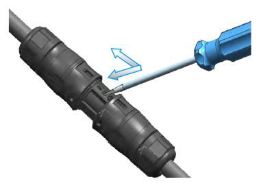
7.4. If the connector to be disassembly for rewire, please according to the following steps:
