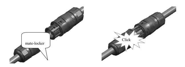
7.3. If the connectors are separated, choose a corresponding flat screwdriver to push mate-locker step slightly out of position, and then give a force along the axial direction until separation.
