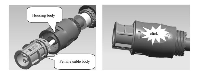
6.3.4. Push the sealing body and sealing craw into the housing body, and then tighten the end locker, torque  $4.0\pm0.5N\cdot m$ .
